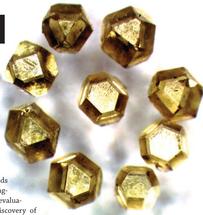
ABOVE Synthetic diamonds recovered after caustic fusion process illustrating the absence of corrosion on diamond surfaces
