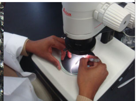
ABOVE Sorting residue after caustic fusion for diamonds using a 60X binocular microscope
